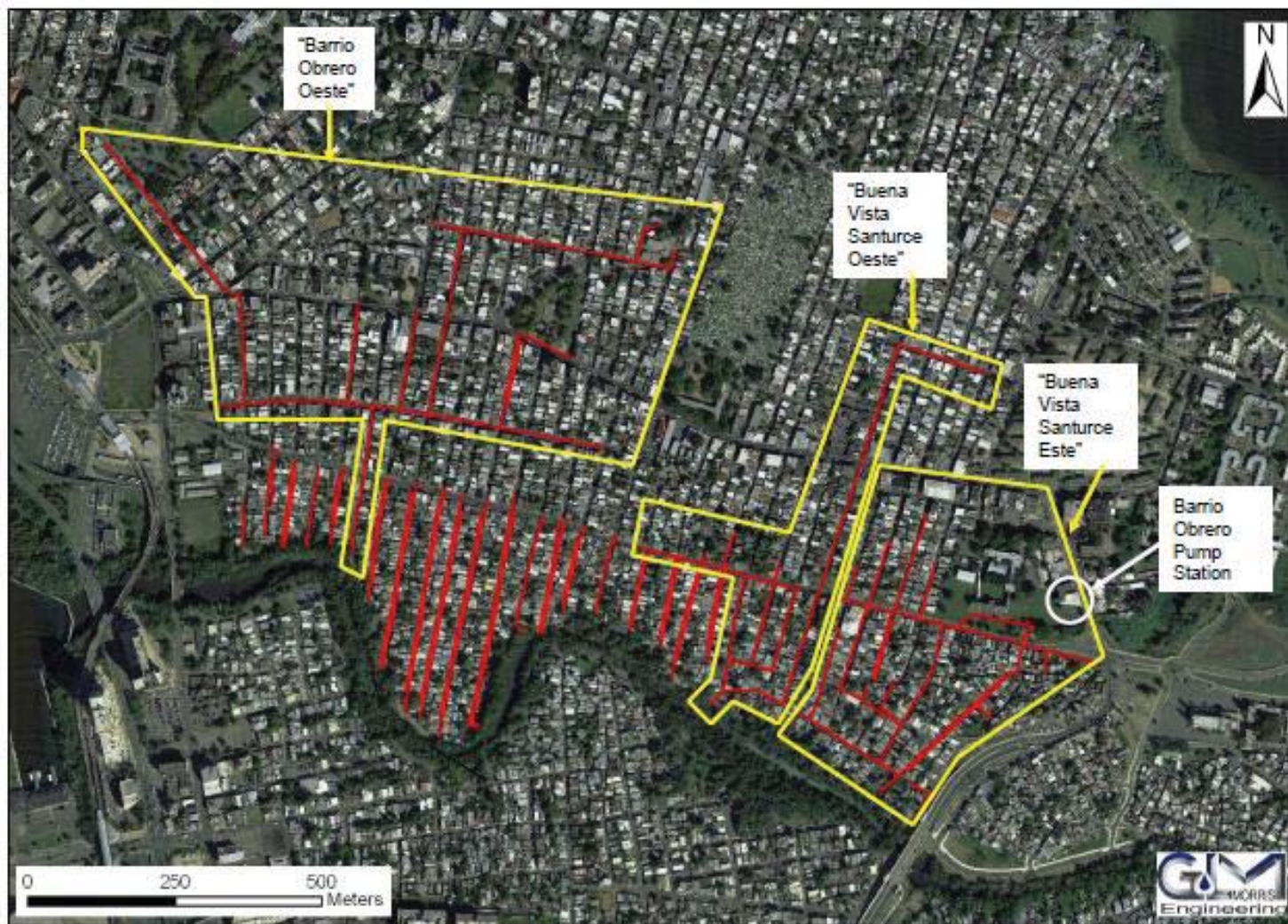
Figure 4.2-3. Existing Storm Sewers North of CMP
