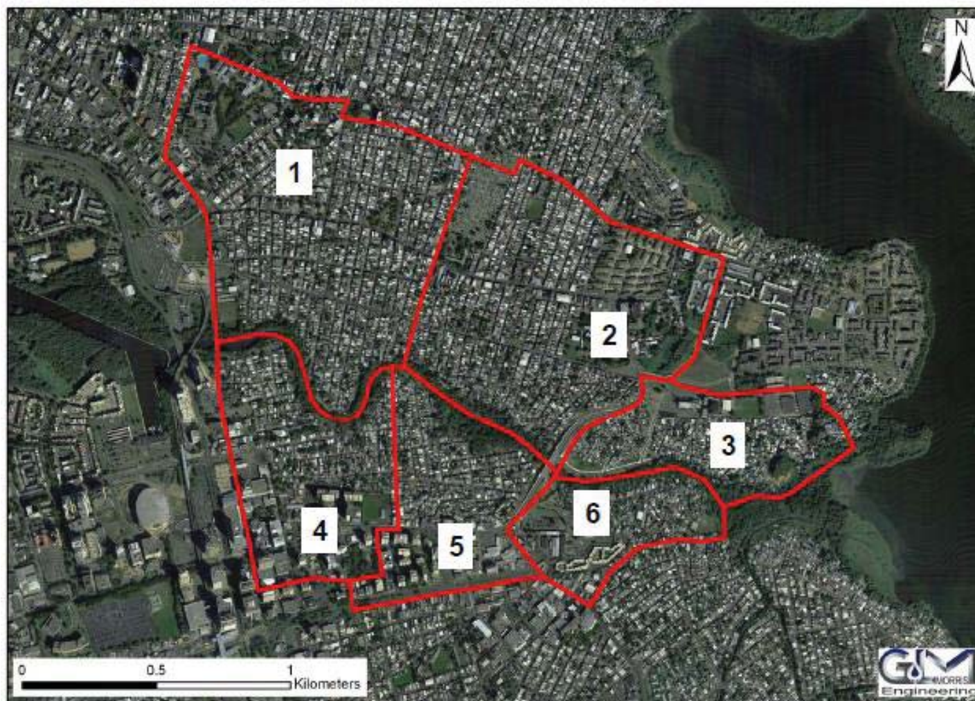
Figure 4.2-2. Watershed Limits for areas draining into CMP east of Ponce de León Avenue
