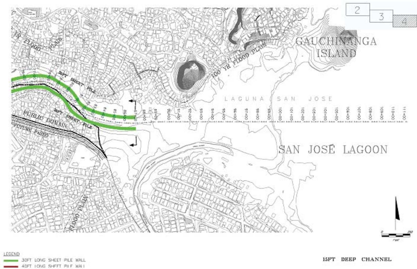
Figure 5.4-8. Sheet Pile Wall Layout, 15-foot-deep Channel
