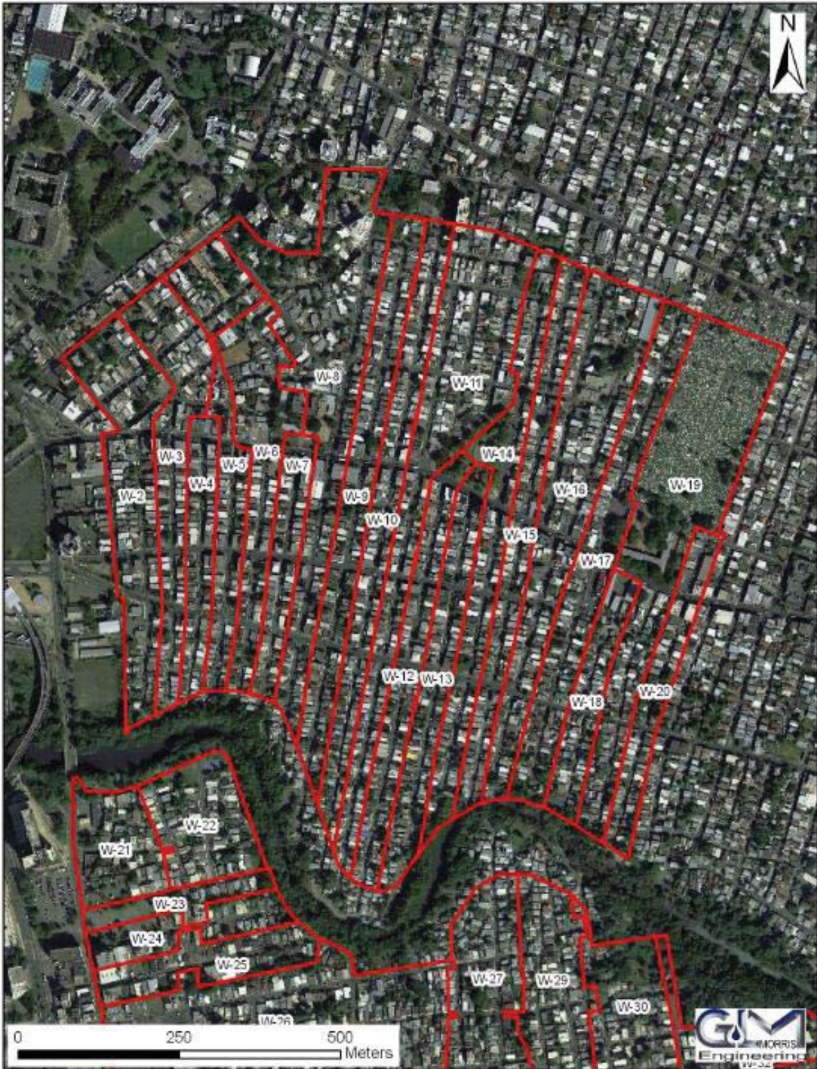
Figure 4.2-7. Drainage Areas North of CMP used in interior drainage analysis
