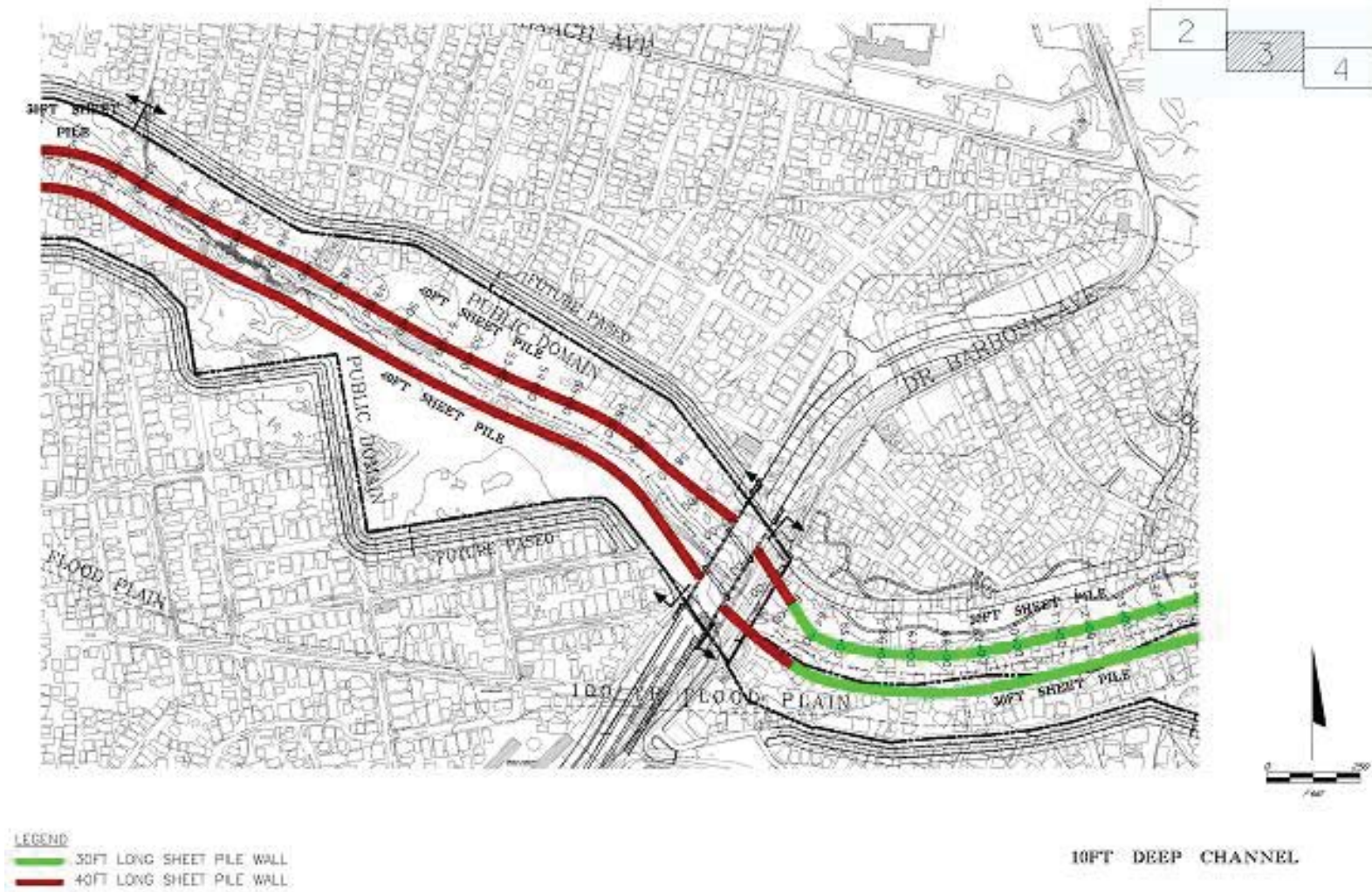
Figure 5.4-3. Sheet Pile Wall Layout, 10-foot-deep Channel
