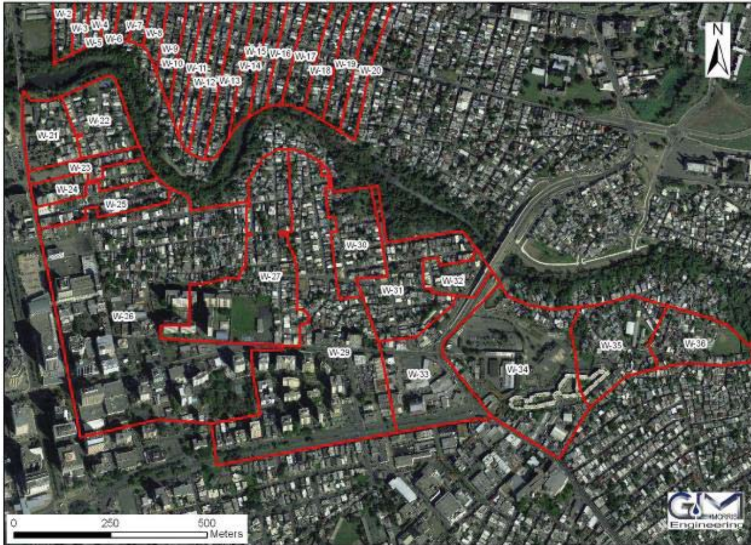
Figure 4.2-8. Drainage Areas south of CMP used in interior drainage analysis
