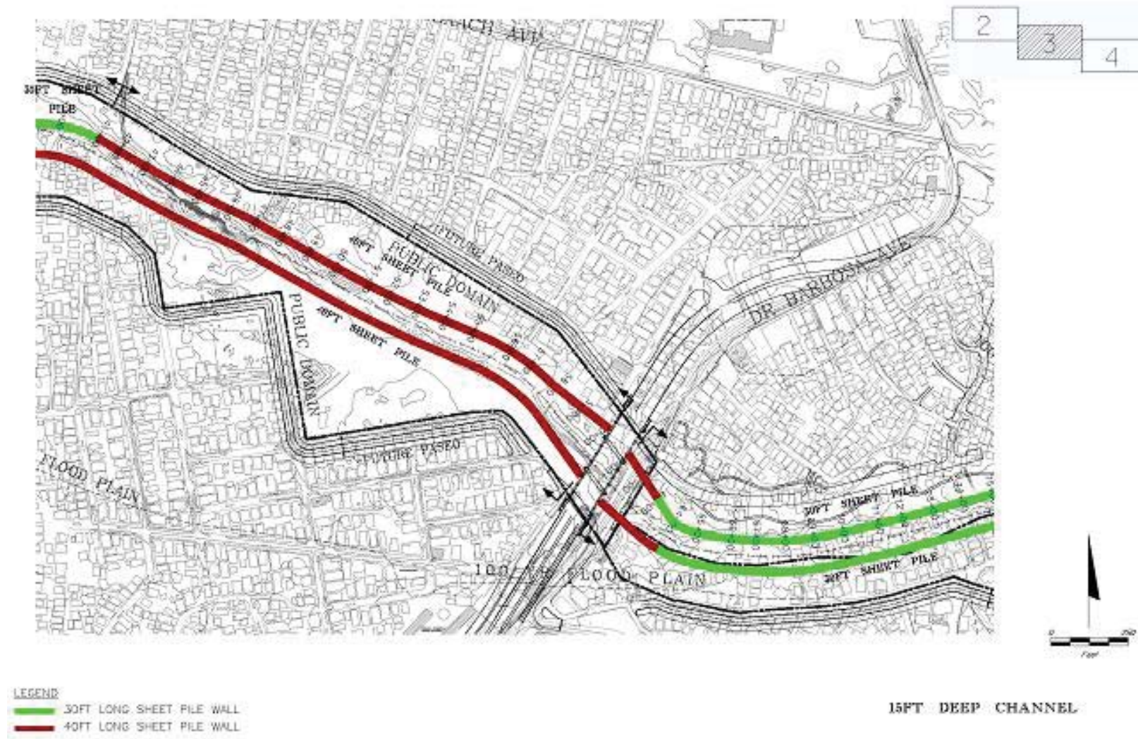
Figure 5.4-7. Sheet Pile Wall Layout, 15-foot-deep Channel
