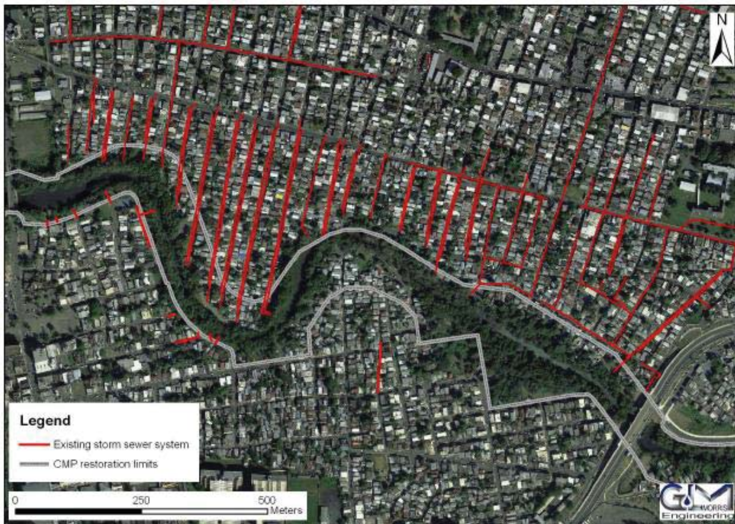
Figure 4.2-6. Portion of Existing Storm Sewer Affected by CMP Restoration
